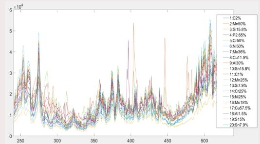
At least 10,000 LIBS spectra from each sample (1064nm Nd:YAG laser, 16ns pulse, 240-518nm spectral window, 0.5μs delay, 20 μs integration time) have been obtained.
