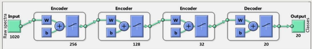
The network has been trained with 5,000 raw spectra from each ingot, preserving the intrinsic shot-to-shot intensity variations. The classification performance with **new spectra not used for training** shows a 0.3% classification error.
