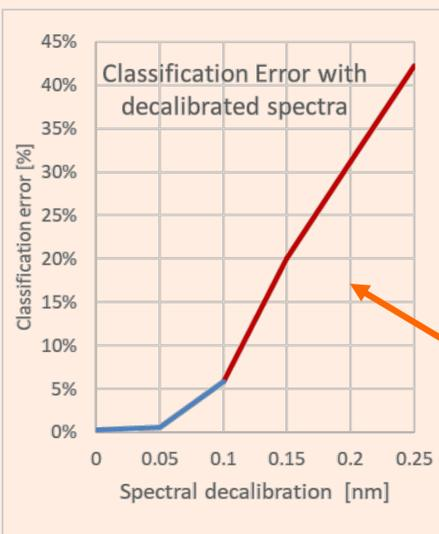
However, the **expected long-term wavelength decalibration** of the spectrometer should affect the classification performance (+/- 0.25nm deviation for a 10°C temperature change has been reported). The measured spectra have been artificially decalibrated and the robustness of classification has been obtained.
