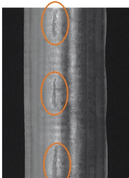
Figure 4. Surface marks due to broken rolling stands
