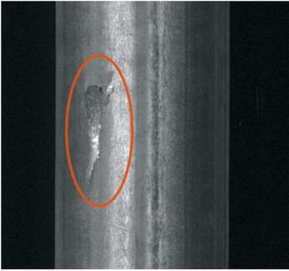
Figure 3. Surface defect: lack of material
