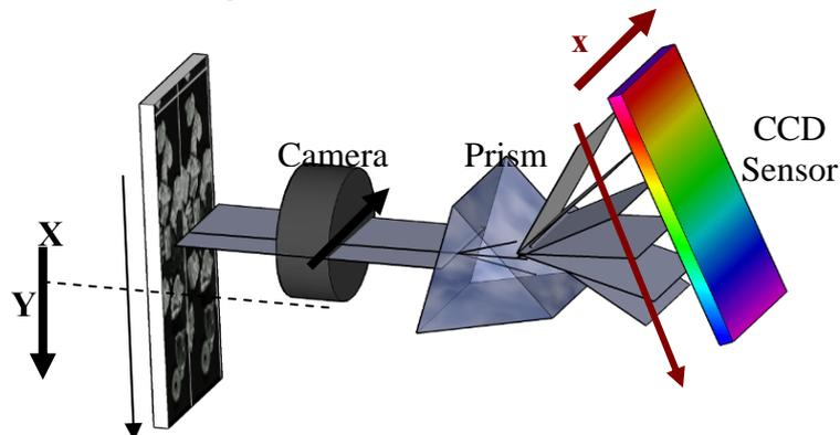
Fig. 2 Principle of hyperspectral image capture.
