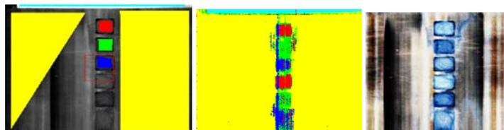
*Fig. 6 Classes created, classified sample and with pseudocolored balanced lighting. The chosen wavelengths for colouring have been 1121 nm, 1494 nm and 2319 nm.*
