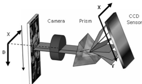
Fig. 2. The hyper-spectral image acquisition process.
