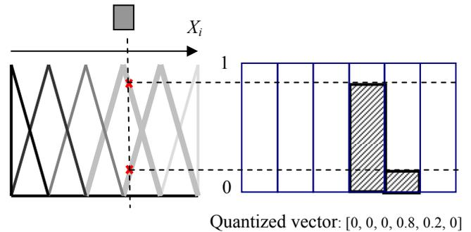
Fig. 10. The fuzzy-based vector quantization procedure. This diagram illustrates the calculation of the quantized vectors when 6 fuzzysets are employed to sample the hyper-spectral domain.
