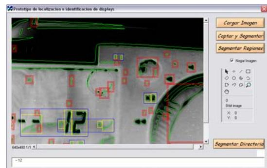
**Figure 11. Video display image and its processing.**
