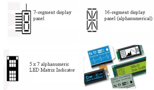
**Figure 2: left to right, top to bottom, 7 segment, 16 segment, dot matrix and graphics display panels.**
