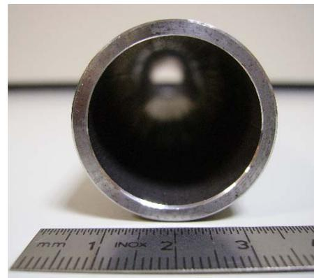
Fig. 1. Example of tube with bevel
