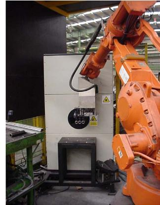
Fig. 18. Robot and gripper in the inspection location
