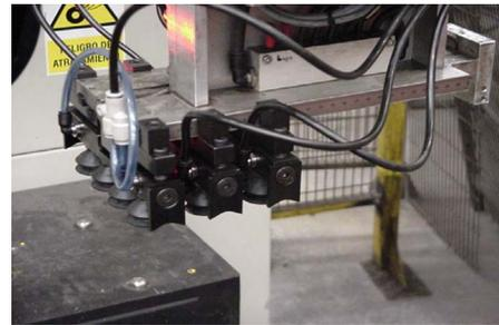
Fig. 19. Vacuum gripper
