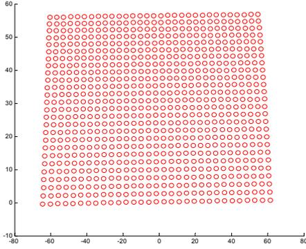
Fig. 10. Conversion Results from a square matrix of points belonging camera reference system into laser plane reference system.
