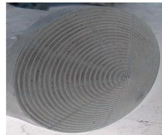
Fig. 9. calibration element, used to calculate the coefficients of the camera2plane conversion function
