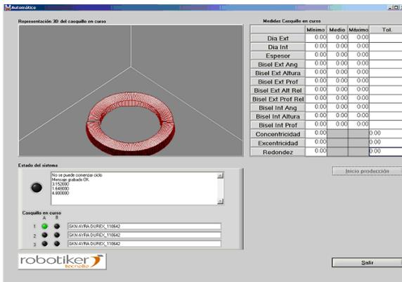
Fig. 21. Automatic inspection user interface.
