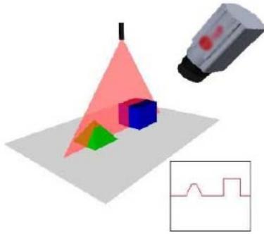
Fig. 2. Triangulation principle [3]
