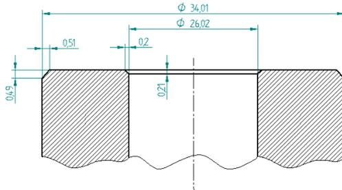
Fig. 16. Some Measures obtained from the tube
