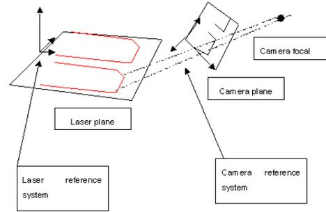
Fig. 8. Relation between inspection camera reference system and laser plane reference system.
